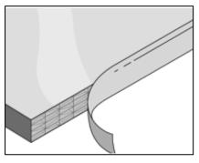
Aluminium foil adhesive tapes are used in order to seal the heads of MACROLUX® MULTIWALL sheets, so that dust will not get within the chambers. However, they should contribute to ventilation within the chambers, so that the water transmigrating due to hygroscopicity can evaporate easily.
