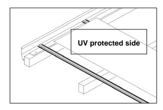
**D.** Position the sheets, to which the aluminium tape has been applied, MAKING SURE THAT THE UV-PROTECTED SIDE (recognizable through the coloured film and the branding made with a hot instrument) IS FACING OUTSIDE.
