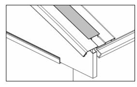
J. Insert the cap (cod. M9T1) required for correct finishing and to hide the fastening screws.
