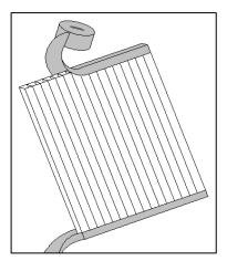
Prior to setting up, the heads of MACROLUX<sup>®</sup> MULTIWALL sheets should be closed with adhesive aluminium tape in order to preserve the cleanliness of chambers over time.
