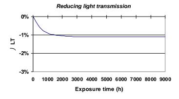
The UV protection limits to the range of a few percentage points the loss of light transmission for MACROLUX® MULTIWALL sheets in the course of time.
