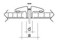
In order to fix MACROLUX® MULTIWALL sheets with passing screw, buttons which allow the user to achieve the necessary mechanical reinforcing
