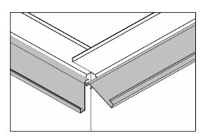
C. Cut the revolving sill (cod. M9R7) required for the gable, 30 mm longer than the external width of the edge beam. Insert the revolving sill (cod. M9R7) both into the gable and laterally, making sure that the latter protrudes by 35 mm in relation to the edge of the fixed sill.
