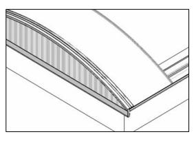
K. Insert the clip for 10mm thickness (cod. M9R4), cut to a length equal to the external width of the edge beams (L) + 200 mm.
