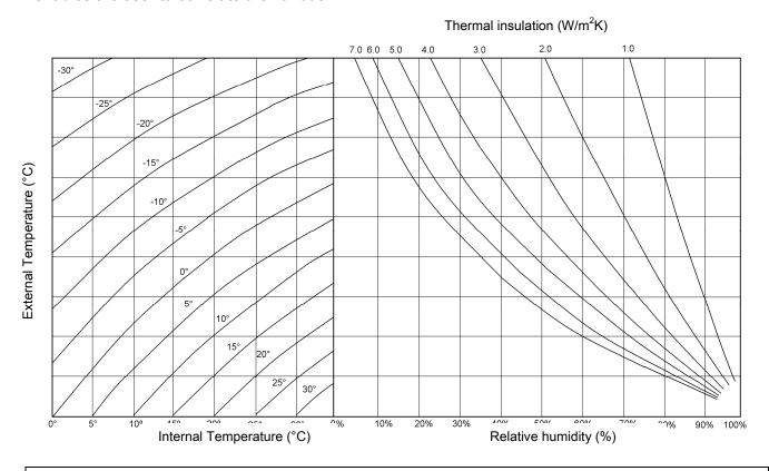
**EXAMPLE:** Checking at which outdoor temperature there is formation of condensation, for a simple glass (U1 = 5 W/m2K) and for a sheet of 16 mm thick polycarbonate 5 W (U2 = 1.9 W/m2K), with relative humidity equal to 60 % and an indoor temperature of 20 °.
