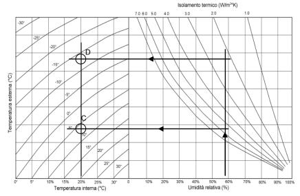
Once the intersection point between the Ur 60% line and the given thermal insulation values (point A and point B), the points (C) and (D) can be found by reading the intersection with the vertical line (internal temperature 20°C).
