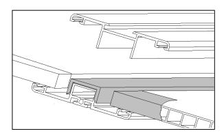
**E.** Fix the sheet with the upper profile, taking care to check that the gaskets are pressed correctly. The joining screw between the lower and the upper profile should be positioned at a distance not exceeding 500 mm..
