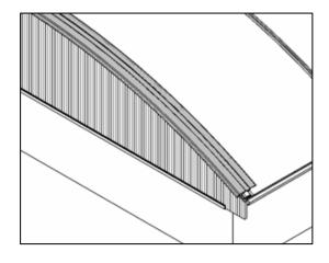
H. Position the upper profile for the gable (cod. M9S9), with the sealing joints in contact with the MACROLUX® MULTIWALL sheet.
