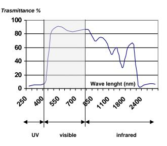
The response to the solar radiation spectrum evidences how a UV-protected polycarbonate sheet can screens the ultraviolet component completely (on average only 4% of the radiation range between included in the nanometers can pass through the sheet), while it remains totally transparent to visible component.
