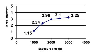
Example of an accelerated aging test in QUV with UVA 340 lamps for 10mm multiwall sheets. The terms and methods for the evaluation of yellow index are detailed in the warranty and in its extension, if one is available.
