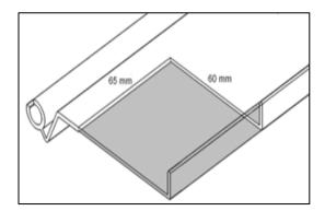
**A.** On the gable side, the sides of fixed sill (cod. M9R6), whose length is equal to the external measurement of the edge beam (L), must be trimmed, cutting away a 65x60 mm section.
