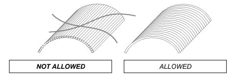
**IMPORTANT:** The cold bending of the sheets must be carried out solely according to the direction of the chambers, a transversal bending is not allowed.
