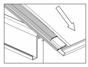
**F.** Insert the thermal cut (*cod. M9T5*) into the lower profile slot.
