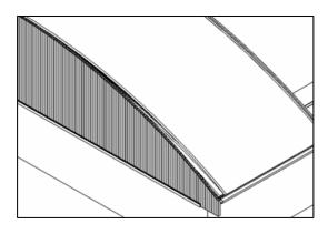
**G.** Cut a 10 mm-thick Multiwall sheet to fill the gable, following the shape given by the upper edge of the gable profile (the ends of the gable sheet must also be closed with the aluminium tape).
