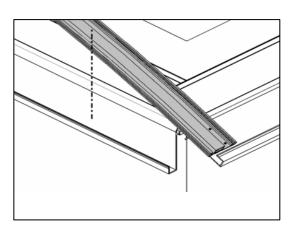
D. Fasten the lower profile of the gable (cod. M9T0) onto the side revolving sill so that the edge of the profile itself is aligned with the gable's vertical sill (cod. M9R7). The profile must be provided with a gasket (cod. M9S3 or M9S5). The lower profile must be calendered to the radius planned in the design. The extension of the profile must be 30 mm less than the extension of the polycarbonate panel.
